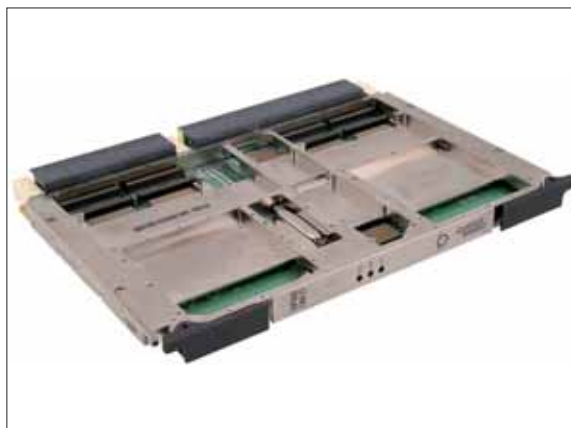
Figure 1. The design of the VPX-185 single board computer will be used for advanced processors that cannot be cooled with typical conduction approaches.
