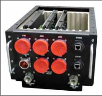
Figure 4. Liquid in the sidewalls is used because of inherently superior thermal properties. (Photo courtesy of Hybricon)
